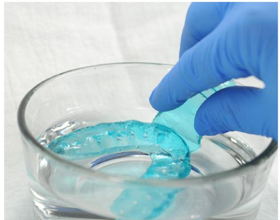
**Note:** Do not leave the part in the alcohol solution for longer than 5 minutes.
