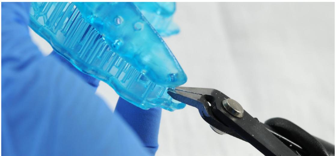
Remove supports using a cutting disk and handpiece, or other part removal tool.
