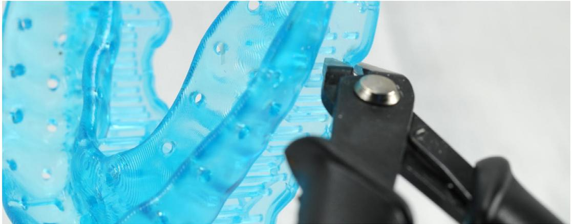
Removing supports should leave a small positive feature.
